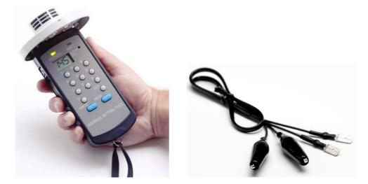
Left: An analog detector is plugged into the address setting tool's snap connectors. Right: Connection cable, to be used when required.
