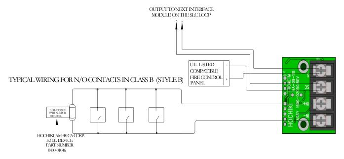
ALL CIRCUITS ARE SUPERVISED AND INHERENTLY POWER LIMITED
